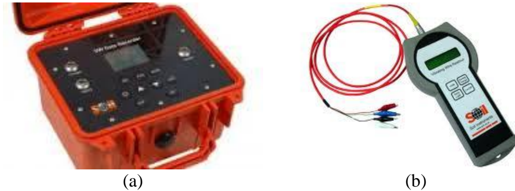
Figure 3-3 : (a) Portable VW recorder (b) Hand Held VW readout unit.
