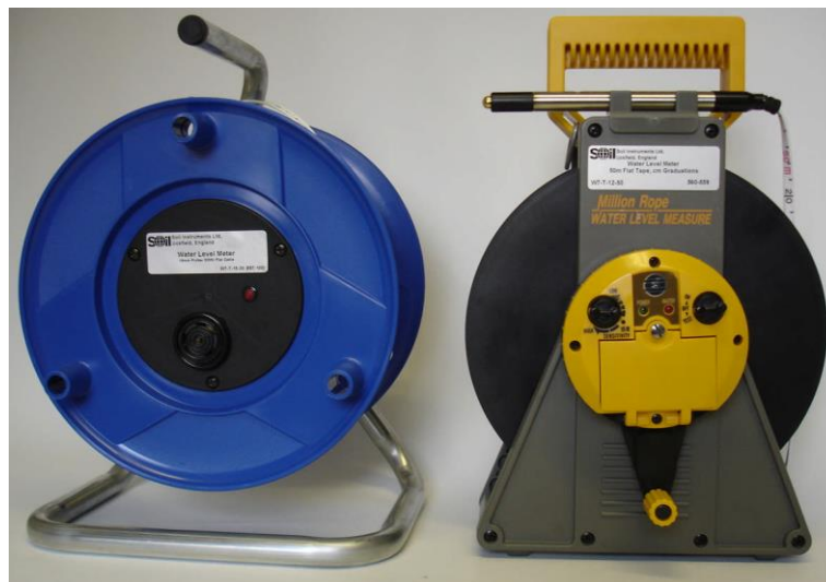
Figure 3-4 : Water Level Indicators.
