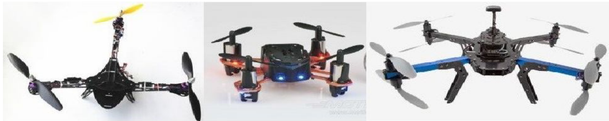
Figure 2.2: From the left to right, tri-, quad- and X octocopter.
