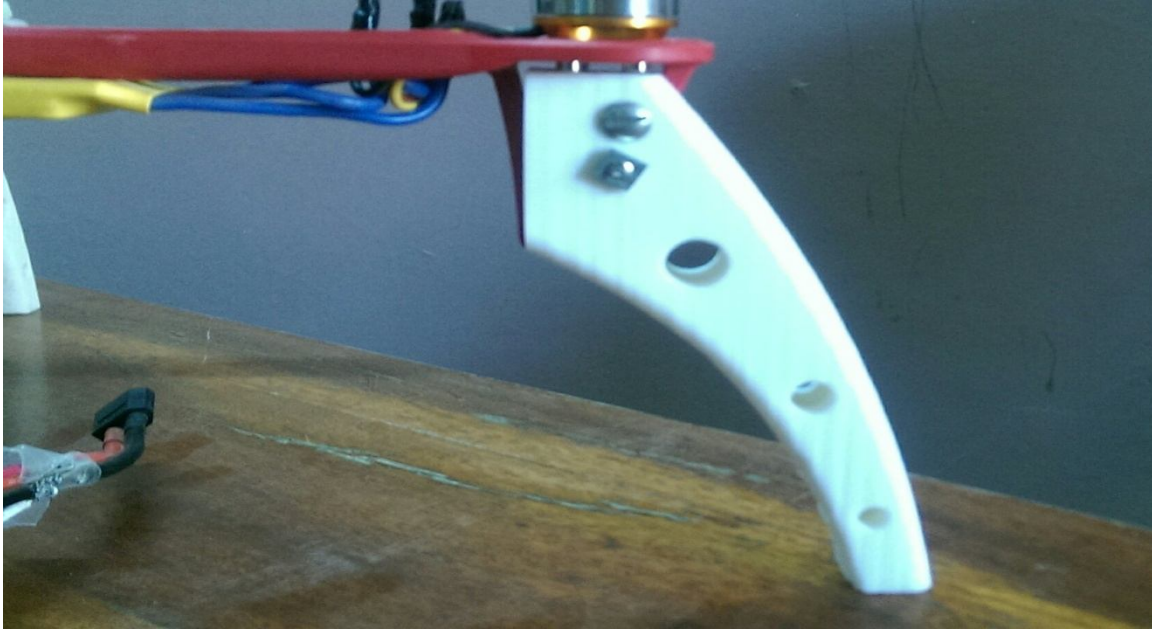
Figure 3.24: Modified Landing Gear to Frame
