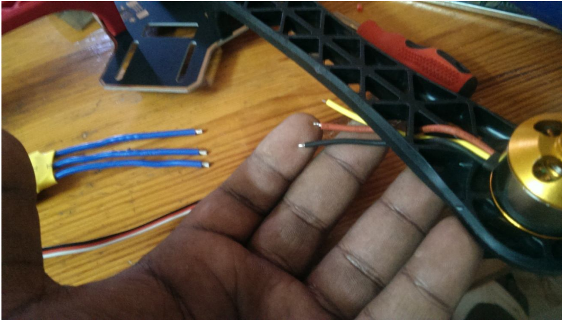
Figure 3.18: Solder Motor to ESC
