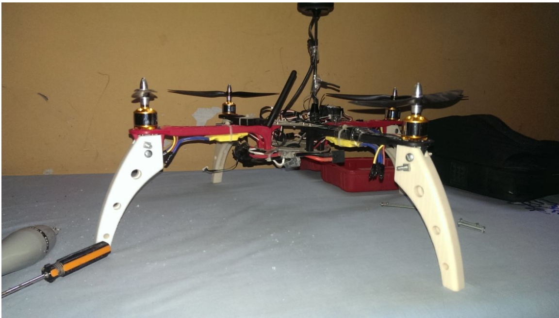
Figure 3.25: Modified Landing Gear to Frame
