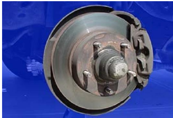
Figure 3.18: The Disc Brake Type [6]
