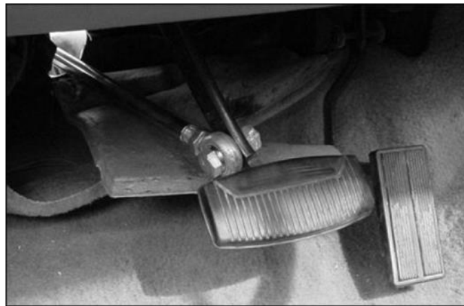
Figure 2.9: Linear brake actuator through firewall
