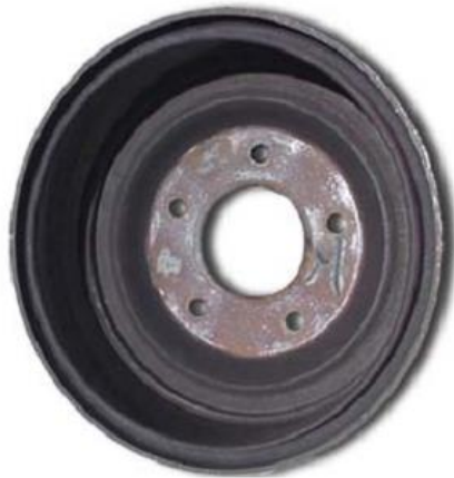
Figure 3.26: The drum brake rotor [6]
