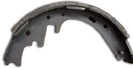
Figure 3.25: The drum brake pads [6]
