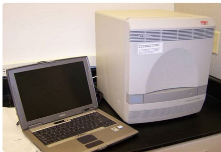
Figure (6.2): RT-PCR (reverse transcription-polymerase chain reaction) is a sensitive technique for mRNA detection
