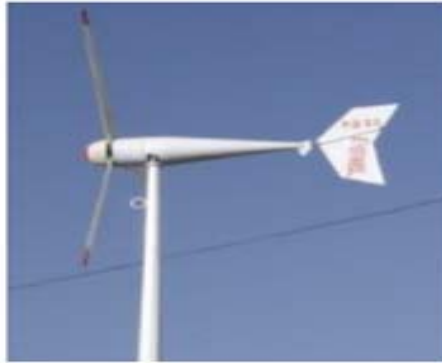
Figure 2.16: Propeller type wind turbine with tail van for yaw control
