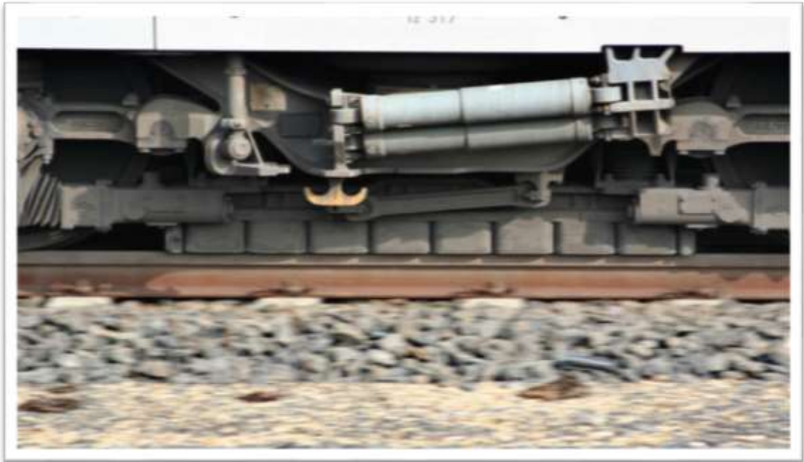
Figure 2.3: An eddy current brake of an ICE 3.
