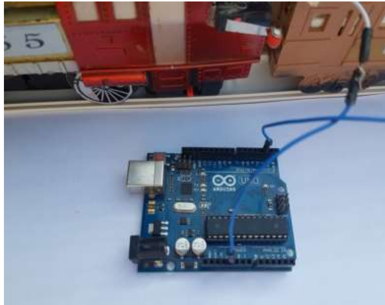
Figure 4.6: Limit switch connected with arduino
