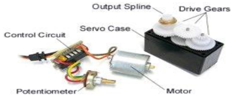
Figure 3.7: Construction of servo motor
