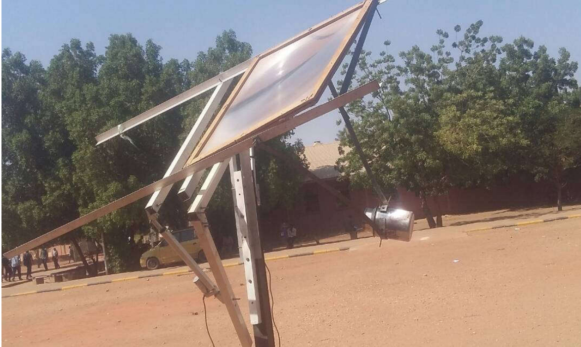
Figure 4.3: Final structure of tracking system with Fresnel lens
