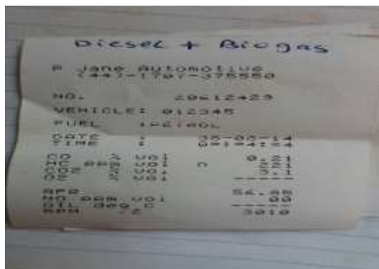
Figure 4.7: Biogas-diesel dual fuel system exhaust gases
