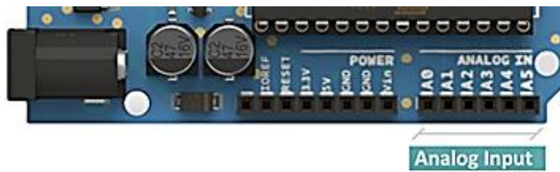
Figure 2.22: Arduino analog pins
