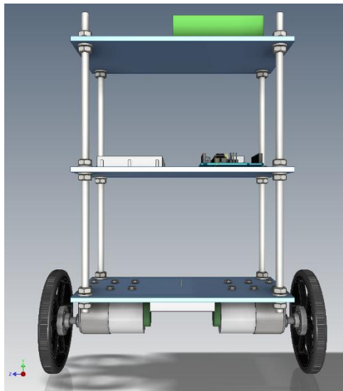
Figure 2.11: Two wheeled self-balancing robot
