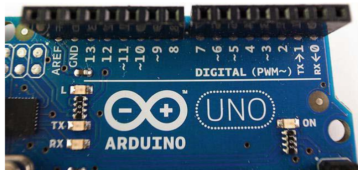
Figure 2.21: Arduino digital pins
