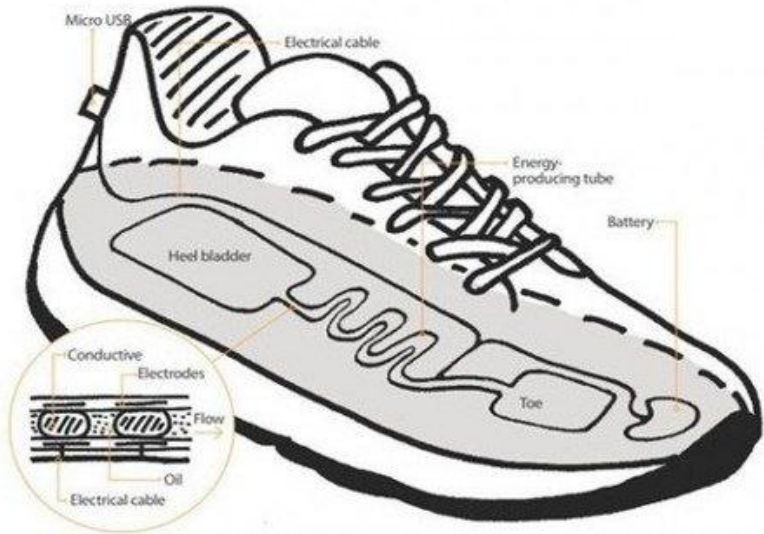
Figure 2.3: the crystal shoe design
