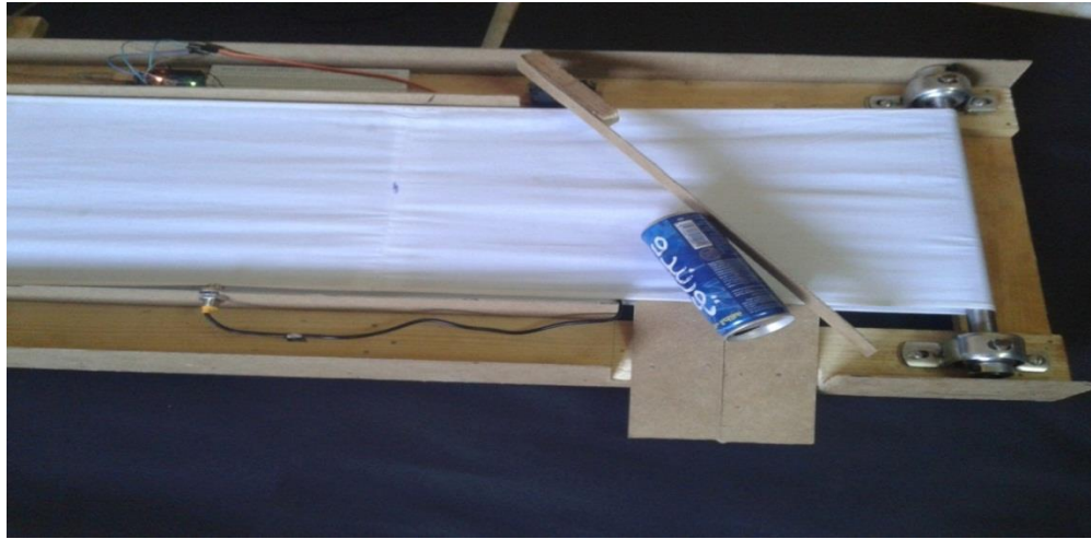
Figure 4.6: The metal material deflected for assignment place
