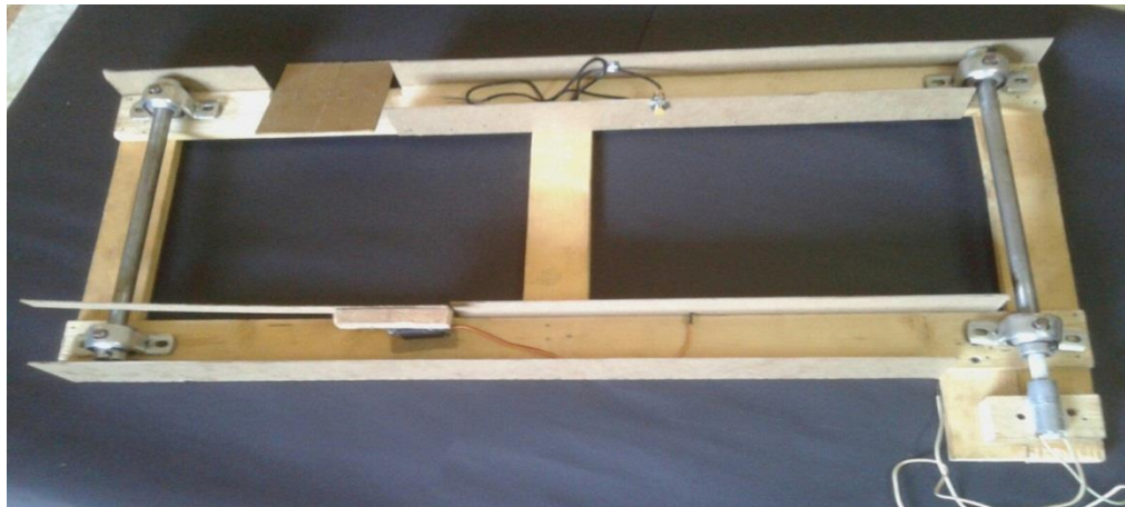
Figure 4.2: The Shaft on chairs and DC motor
