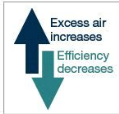
Figure (2-8): Excess air and efficiency relationship
