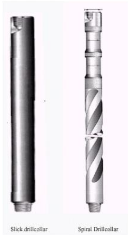
Fig.1.3: Drill Collars Profiles (Well Engineering and Construction, Rabia).
