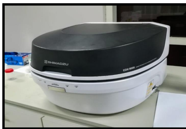
Fig.(3.9): Shimadzu (EDX-8000) X-ray Fluorescence
