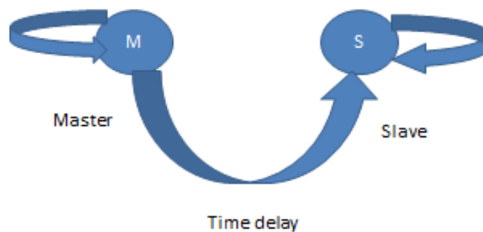
Figure 3.2: Unidirectional coupling Sketch of two delayed laser.
