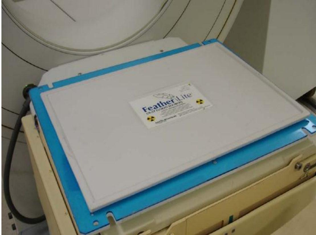
Figure 3-3 gamma camera with a quadratic bar phantom placed on top of the gamma camera detector and radioactive source on top of the quadratic phantom for transmission images.
