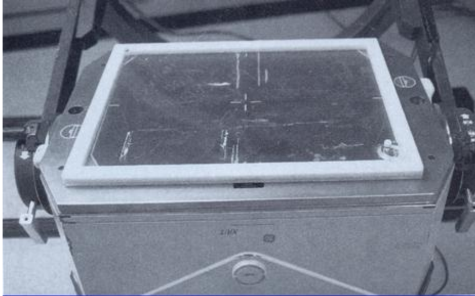
Figure 3-1 an image show a flood phantom covered the face of gamma camera where the phantom filled with ^{99m}\text{Tc} .
