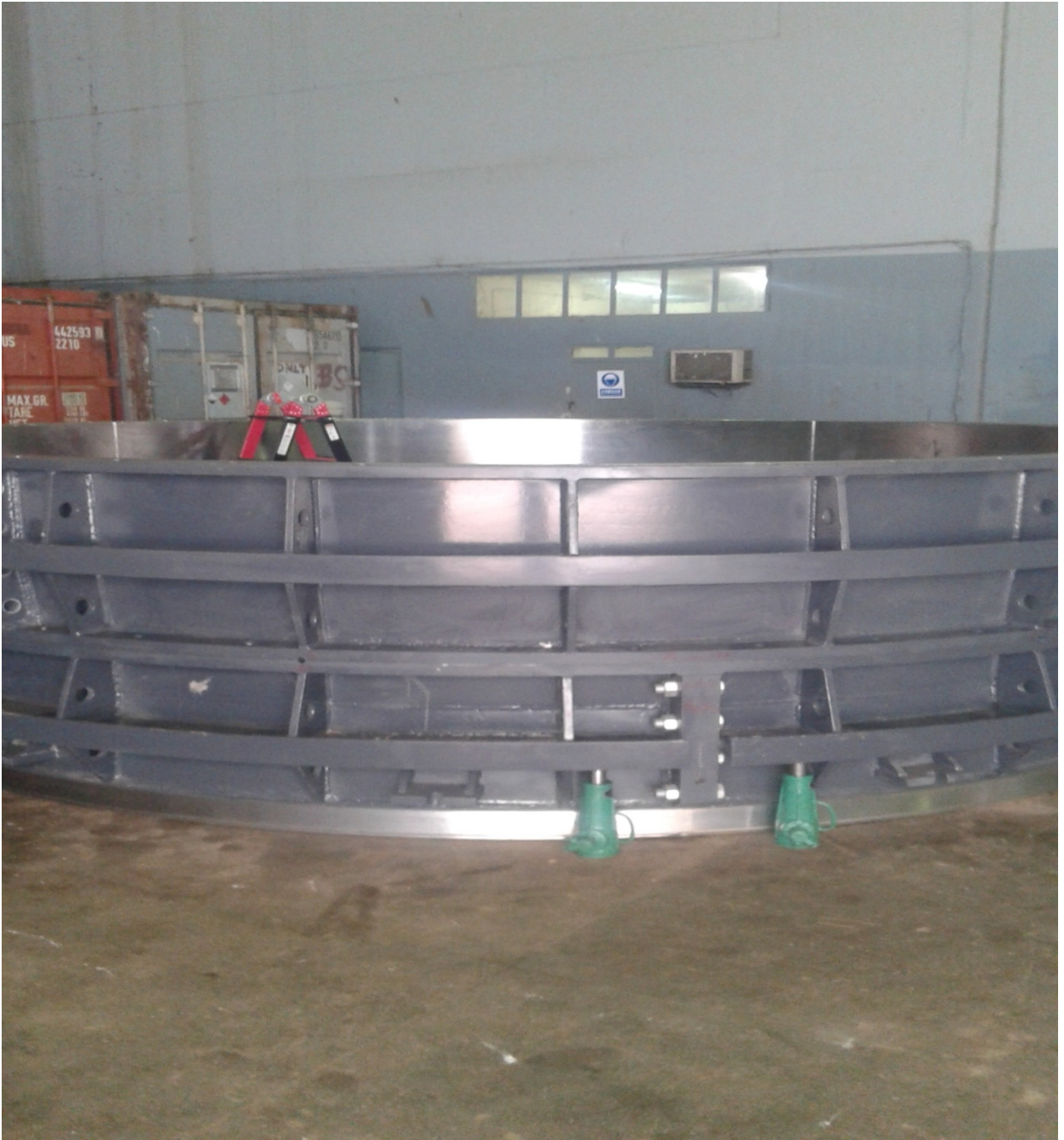
Figure (2.6) The Discharge Ring
