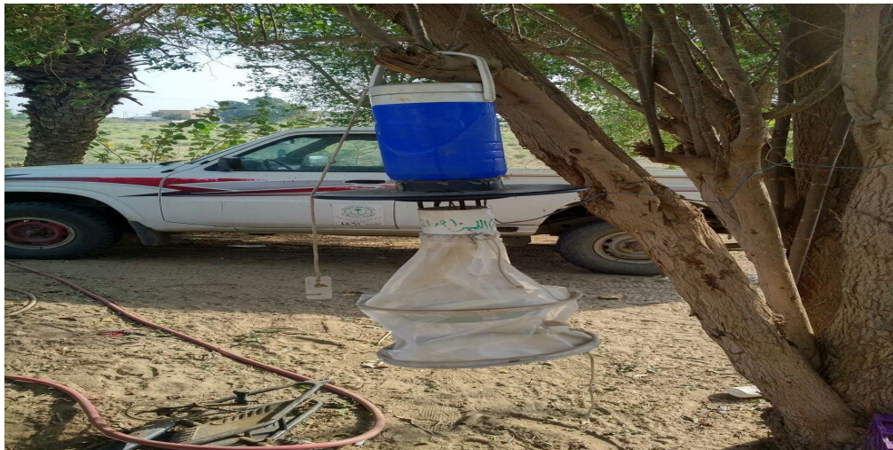
Figure 1.7: \text{CO}_2 baited traps for mosquito surveillance in Jazan region
