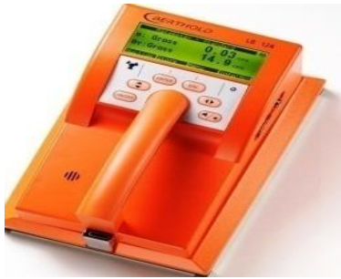
Figure 2.5 shows the contamination monitor LB124SCINT-300
