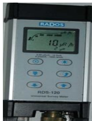
Figure 3.1 shown the survey meter RDS-120.:
