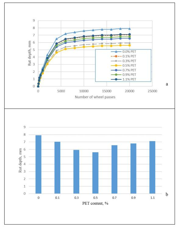
Figure 4 Results of wheel track rut depth
