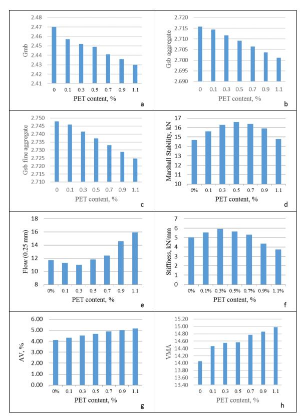
Figure 2: Results of Marshall tests
