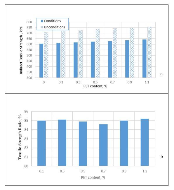
Figure 5 Indirect Tensile Strength tests results of unconditioned and conditioned samples
