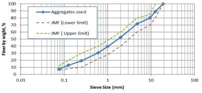
Figure 1: Aggregate gradation
