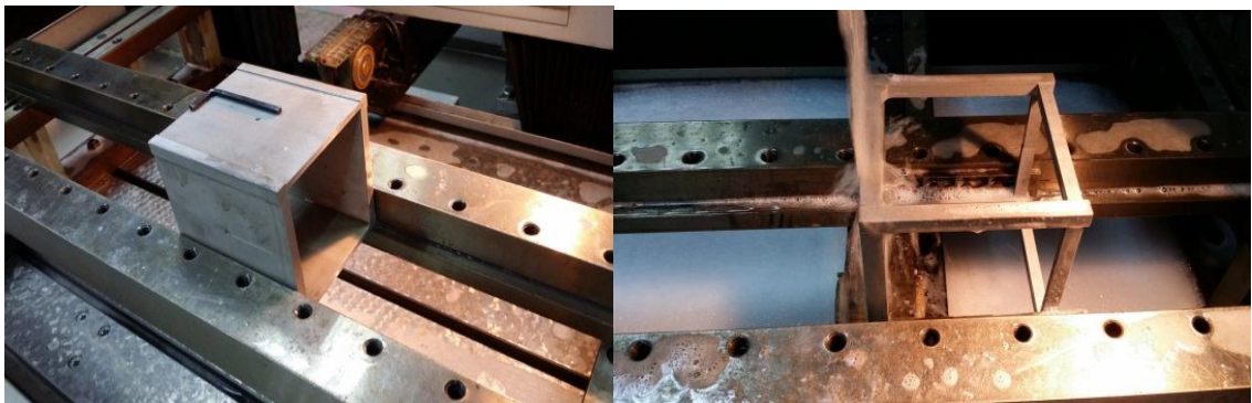
Figure 0-19: processing of the manufacturing in the Wire Cutting Machine.
