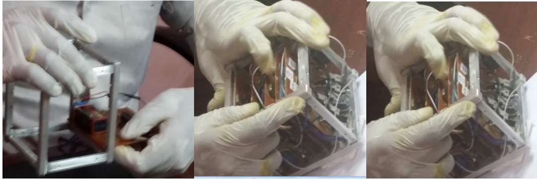
Figure 0-28: ISRASAT1 subsystems attached into the structure.
