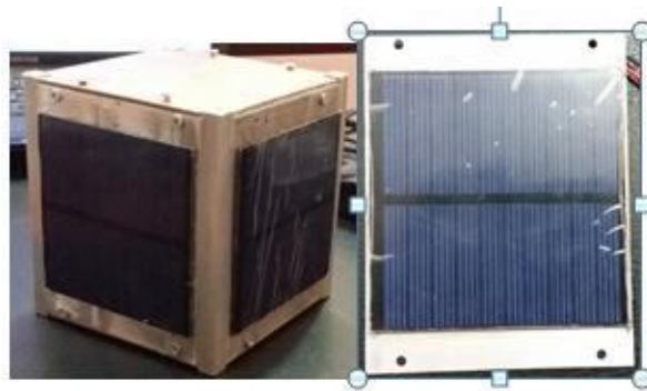
Figure 0-24: Solar Panel Integration.
