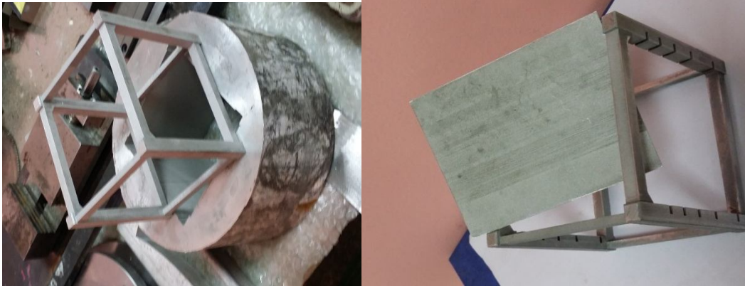
Figure 0-20: final appearance of cube after finished in Wire Cutting Machine.
