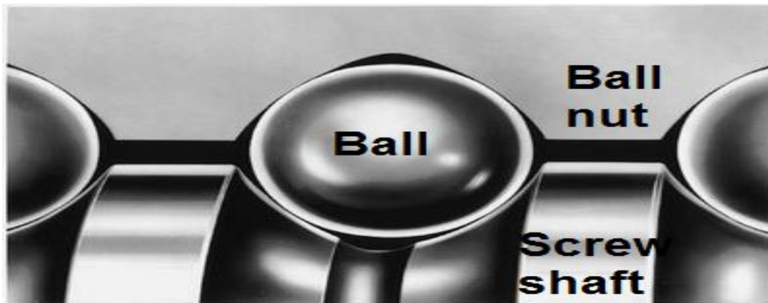
Figure (2.3): Contact between a ball & a ball nut
