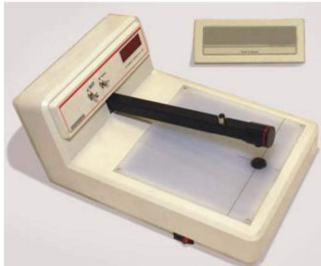
Figure 2.11: Optical densitometer used to measure density on a film.
