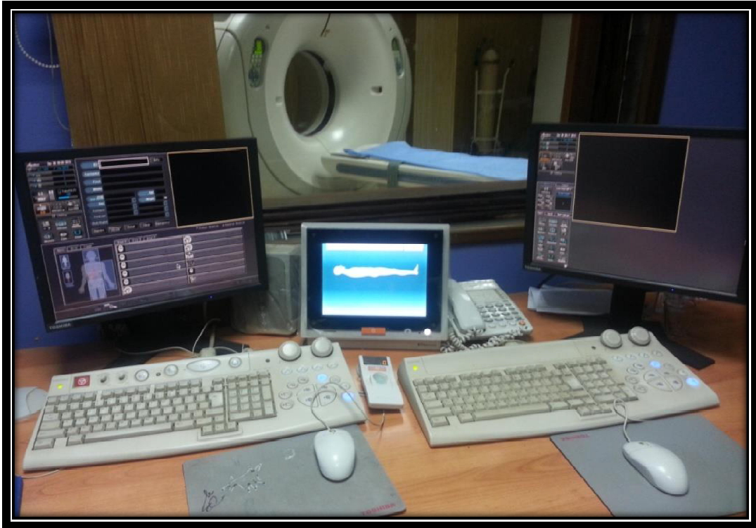
Figure (C1): shows the control panel and monitor of CT machine
