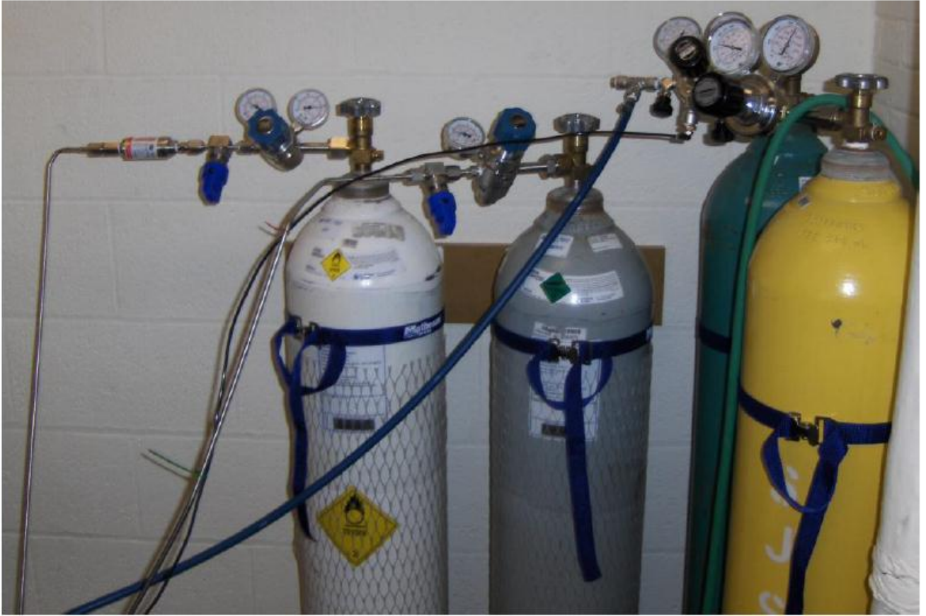
Figure 5.3: Gas tanks (left to right: O 2 , Ar, “low” purity Ar, and Air) and associated hardware.
