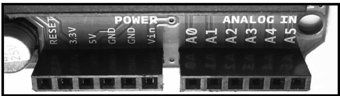
Figure 3.10: The power and analog sockets for arduino uno
