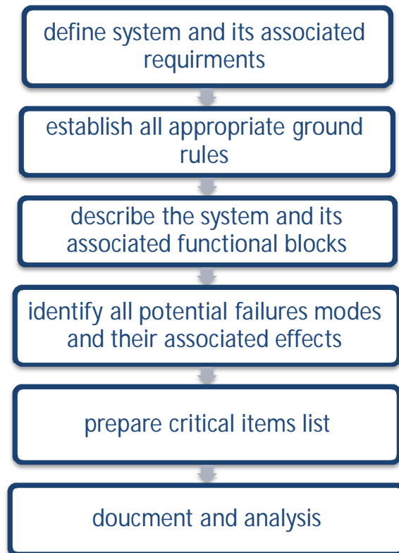
Figure 2.4: Main steps of conducting FMEA [8]
