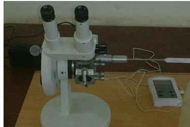
Figure (3.5) photo of the Refract meter
