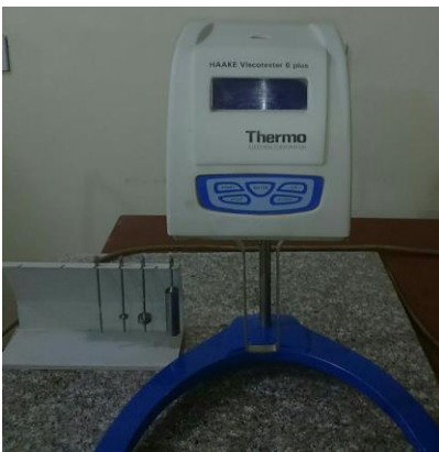
Figure (3.3) photo of the HAAKE Viscometer 6plus
