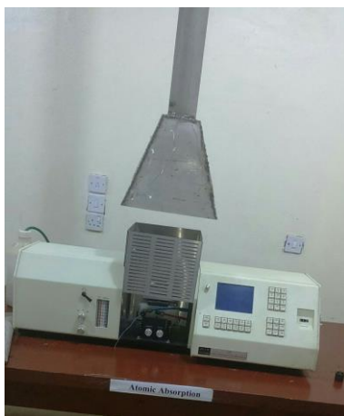
Figure (3.4) photo of the Atomic Absorption
