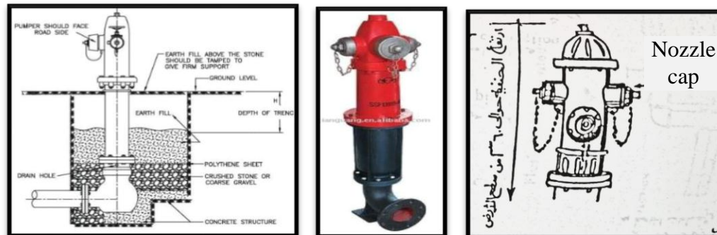
The Figure (3-24) show fire water outlet above the ground. www.arabicsafety.com .
