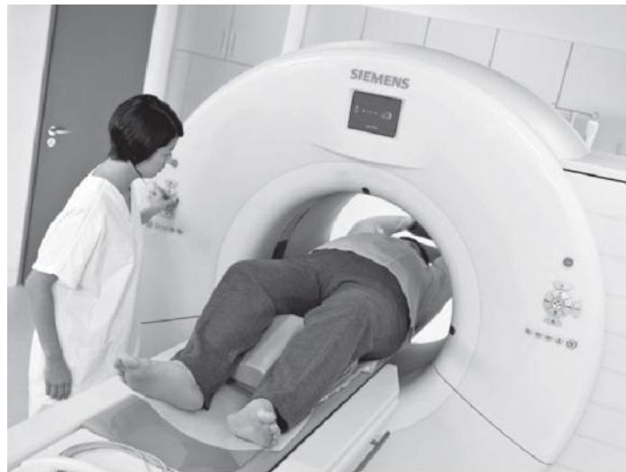
Figure (2.12): CT scanner .The gantry and patient table are Major components of a CT image system. . (Lois, 2011)
