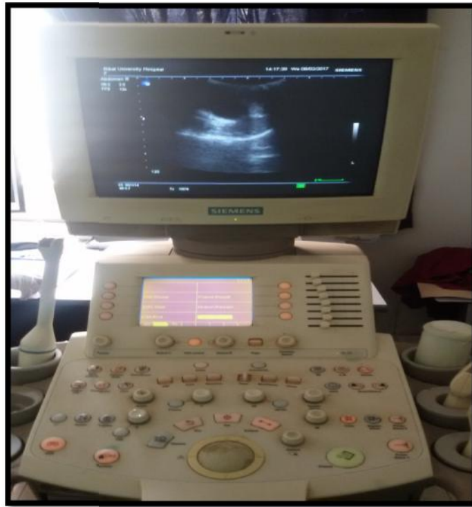
Figure (3-1) Shows equipped with machine(simens, model :MCMD01AA ) equipped with 2-6 MHZ curvilinear transducer which used in this study.
