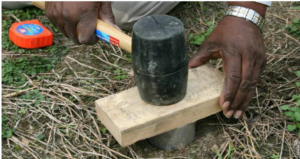
A three inch diameter ring is hammered into the soil to collect bulk density samples.
