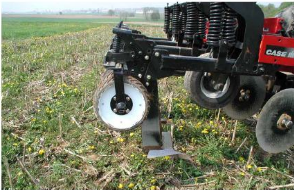
Figure 16: Two types of modern subsoilers that break through subsoil compaction while conserving surface residue cover. (Source:GIZ\Weber(2005))
