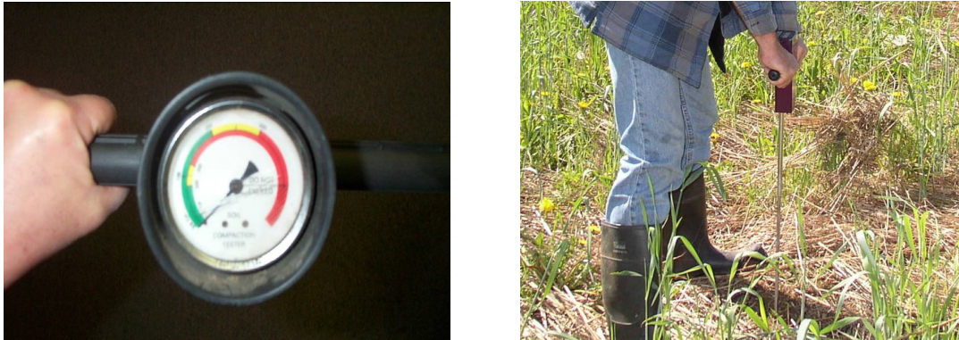
Figure 17. Field penetrometer pushed through the soil profile
