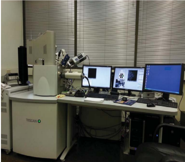
Fig 3-9 Photograph of FE-SEM and EDS systems used in this work.
