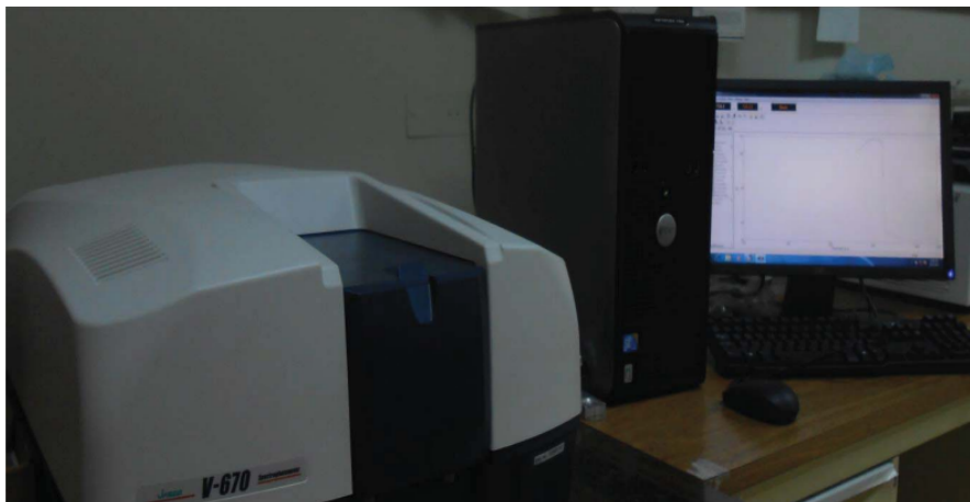
Fig 3-10 Photograph of UV-Vis spectrophotometer used in this work
