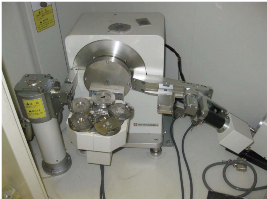
Fig 3-8 Photograph of the X-ray diffractometer used in this study.
