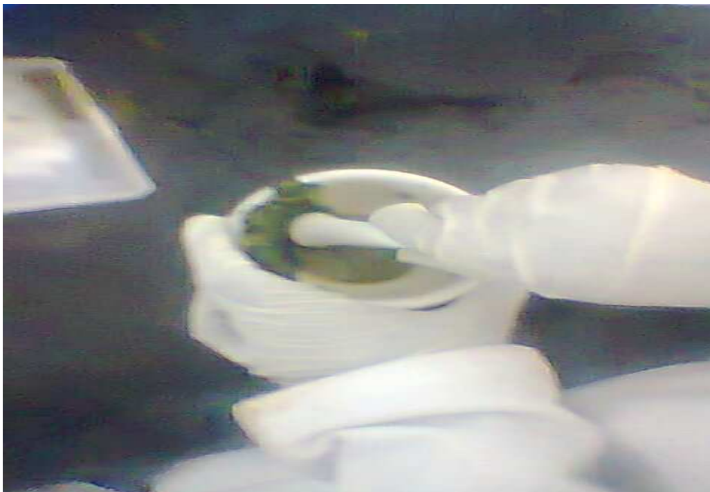
Figure 2: Expressing sap from plant samples by pestle and mortar.
