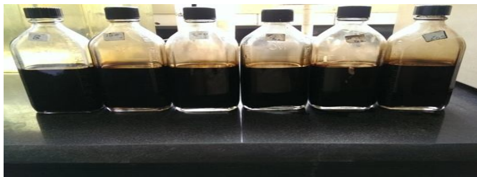
Figure 6 Water separation of HJ.E20 at five different concentrations at 60°C after 24 hours
