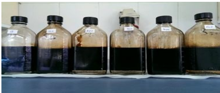
Figure 5 Water separation of HJ.E10 at five different concentrations at 60°C after 24 hours
