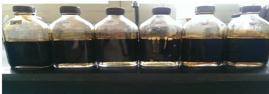
Figure 7 Water separation of HJ.E30 at five different concentrations at 60°C after 24 hours
