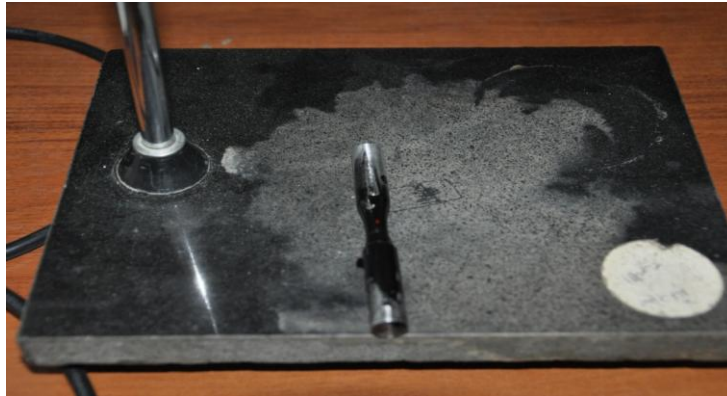
Figure 5: specimen which painted by black paint and then peened.
