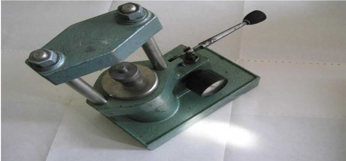
Fig (3.3): A press with a matrix and a punch for pressing of powder of material into a disk.
