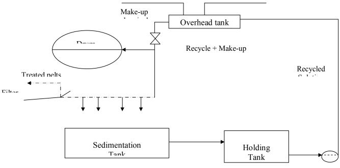
Figure (1): Proposed Recycling of spent solution
