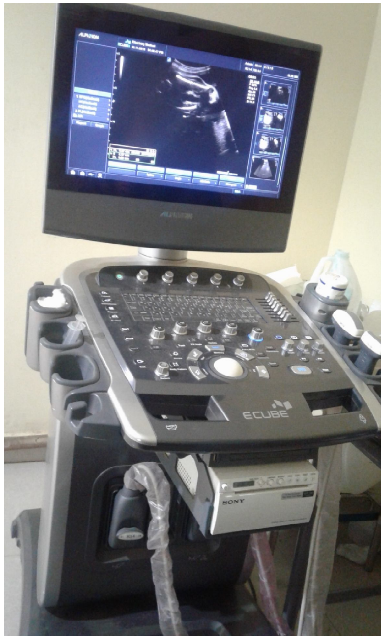
ALPINION 2D ultra sound machine with curvilinear and linear transducers 3.5 and 10 MHZ
