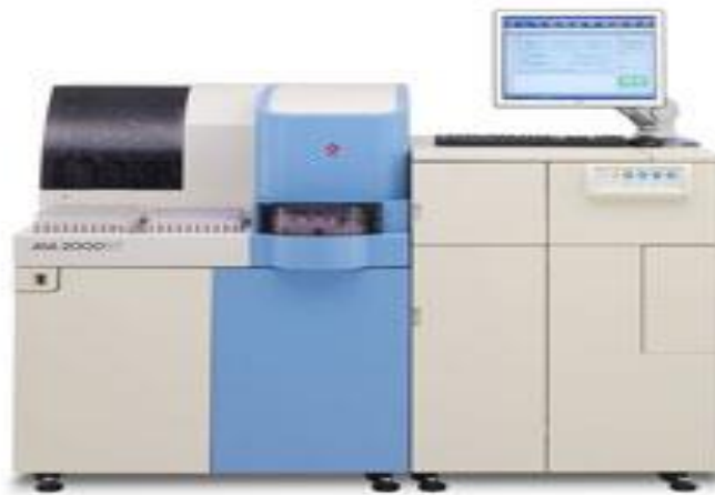
Figure (3.1). Shows TOSOH machine which used in measurement of tPSA and fPSA
