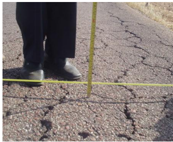
Fig. A.18: High Severity Depression
