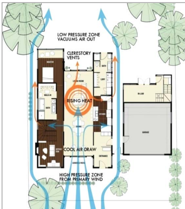
Fig.2.23. Low and high pressure zones plan
