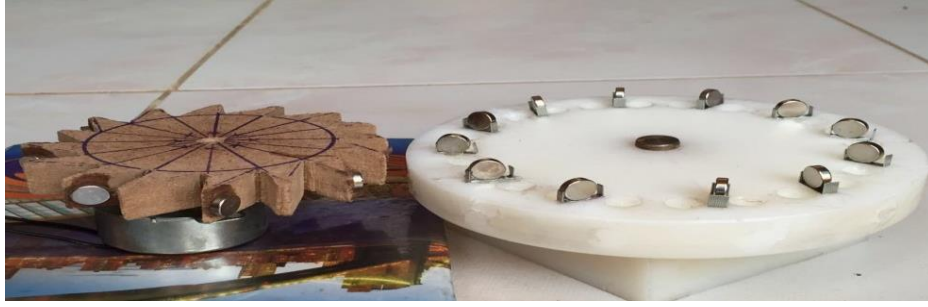
Figure (4.8): Rotor and stator position of condition three
