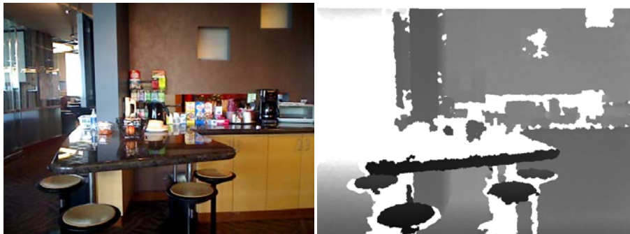
Fig. 2.7 (left) RGB image and (right) depth information captured by an RGB-D camera. [7]
