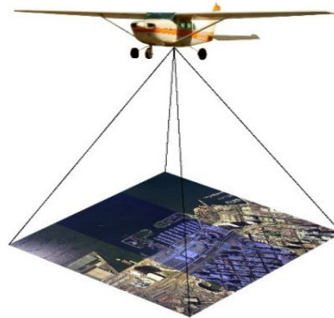
(b) Angular coverage, photo scale and ground coverage of camera.
