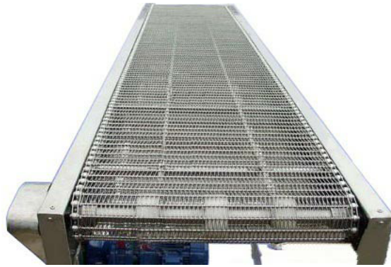
Figure 3.10: Wire mesh belt conveyor
