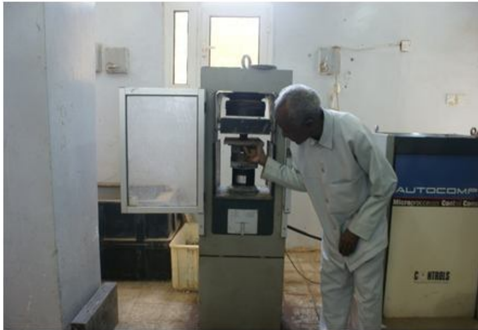
Plate (3.8) Crushing Machine
