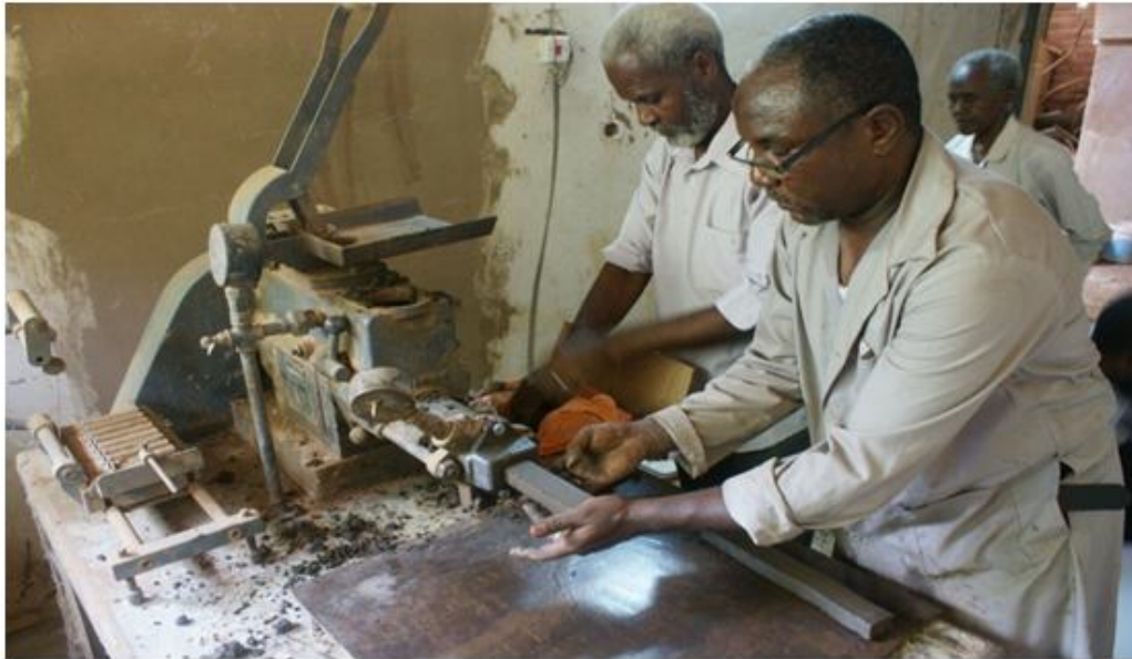
Plate (3.4): Modeling Brick Making M/c
