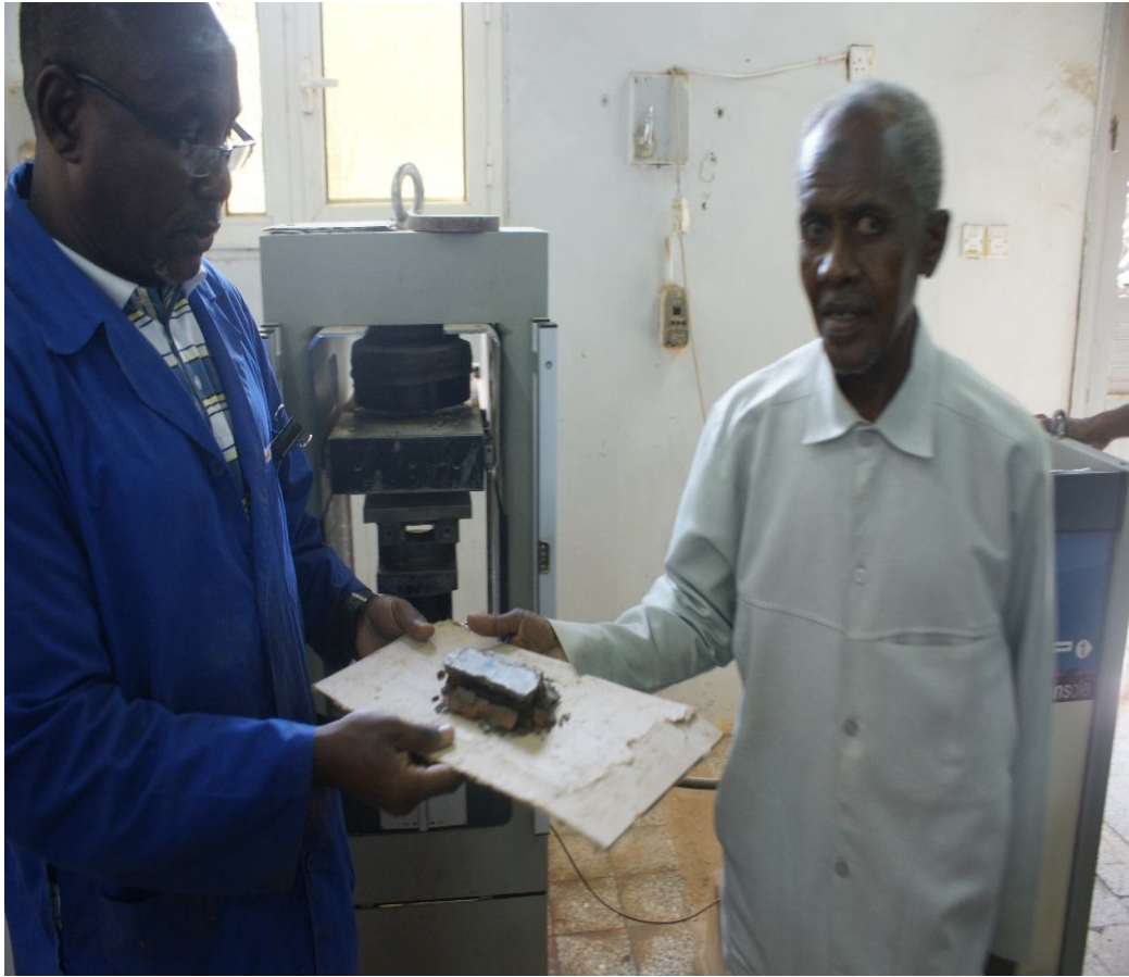
(B-6) Crushing Strength Test
