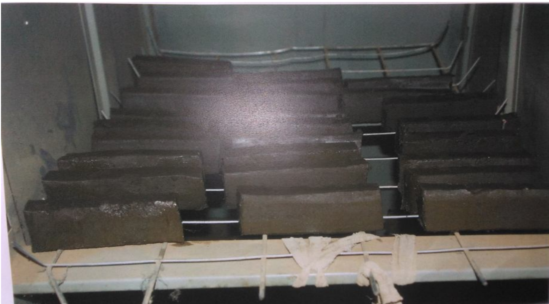
(B- 4 ) Green Brick Drying
