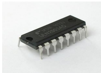
Figure 3.6: Relay driver (ULN2003)
