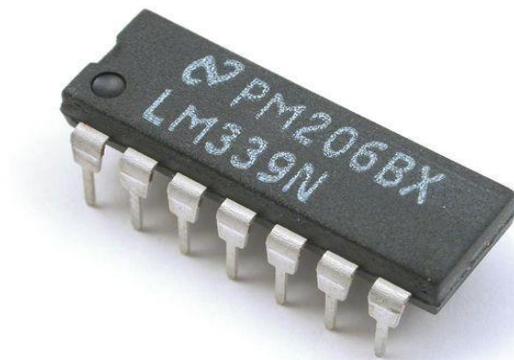
Figure 3.9:Quad Voltage Comparator (LM339N)
