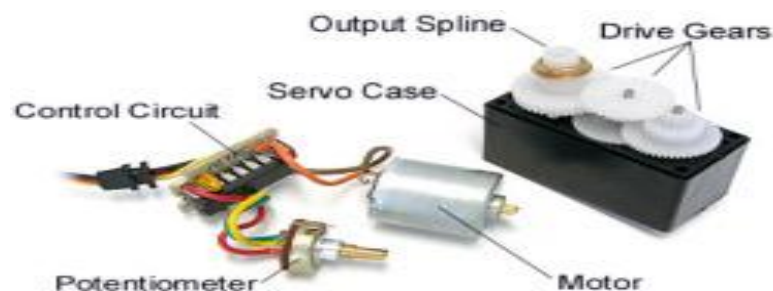
Figure (2.4): The Construction of DC servomotor
